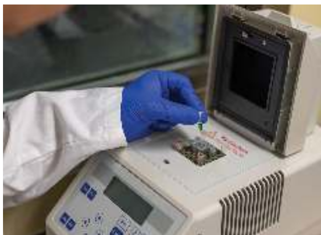
Figure 19.14: Loading a PCR machine (thermocycler) with the reagents needed to amplify small samples of DNA. The machine automatically changes the temperature of the mixtures in each tube. After 30 cycles in this machine there are 2 billion copies ( 2^{30} ) of the original DNA.
