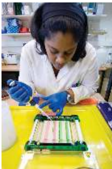
Figure 19.15: Analysing genetic diversity in corals. DNA isolated from coral polyps was amplified by PCR and loaded on to a gel to be separated by electrophoresis.
