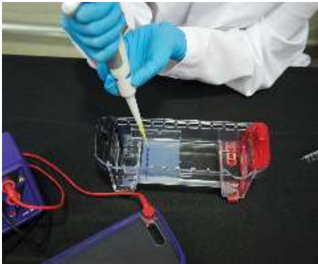
Figure 19.16: Using a micropipette to load the wells in agarose gel with samples of DNA mixed with a blue tracking dye.
